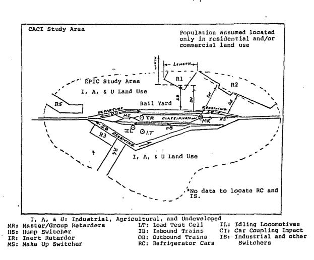
Example of Complex Railyard Configuration -Figure 5. High Volume Hump Yard, Flat Rock Yard, Detroit, MI
